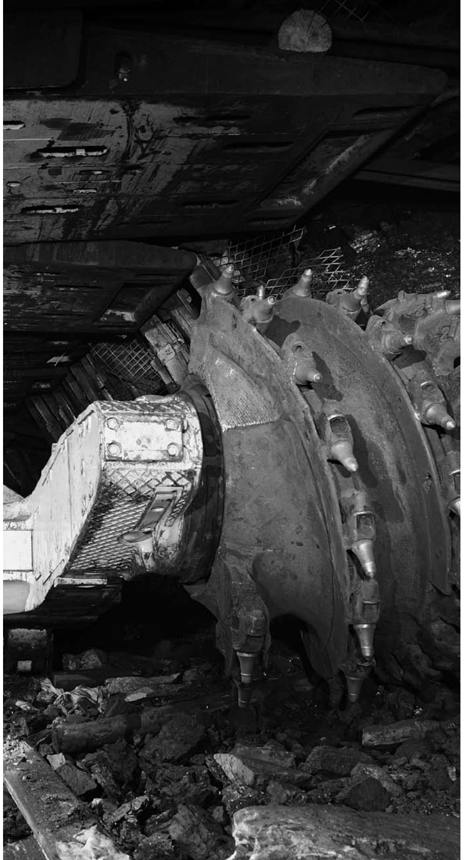
Mid-seam POP 2010 equipment set: conveyor and shearer
