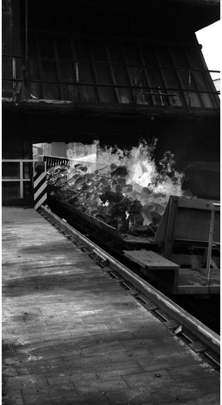
Loading platform of coke-quenching car containing coke with a temperature of approximately 1,100°C
